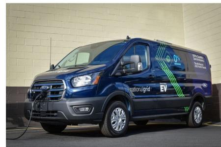
**Ford E-Transit Medium-duty battery electric cargo vans** such as this vehicle run solely on a rechargeable battery. MDVs are class 2b vehicles weighing between 8,501- and 10,000 lbs.
